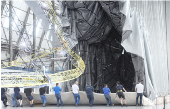
The envelope is pulled over the aluminum and carbon fiber framework of the new airship.
