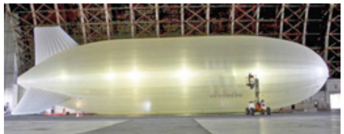
One of the three sizes (versions) of the Hi-Sentinel Airships during inflation test.
