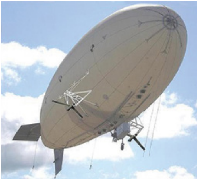
Smaller nonrigid airship carries two Insitu ScanEagle UAS in this concept. Credit: SAIC/ArcXeon
