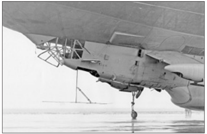
View of the Project Meteor antenna in the extended position seen from starboard. USN/ NARA/Author
